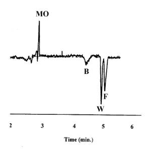
Figure 1. A representative electropherogram obtained with the VACE method. Capillary filled with buffer+ $20\mu$ mol/l BSA+ $100\mu$ mol/l warfarin+ $100 \mu$ mol/l furosemide. Injection solution: 0.067mol/l sodium phosphate pH 7.4+mesityl oxide. MO: mesityl oxide (neutral marker); B=BSA; W=warfarin; F=furosemide.
