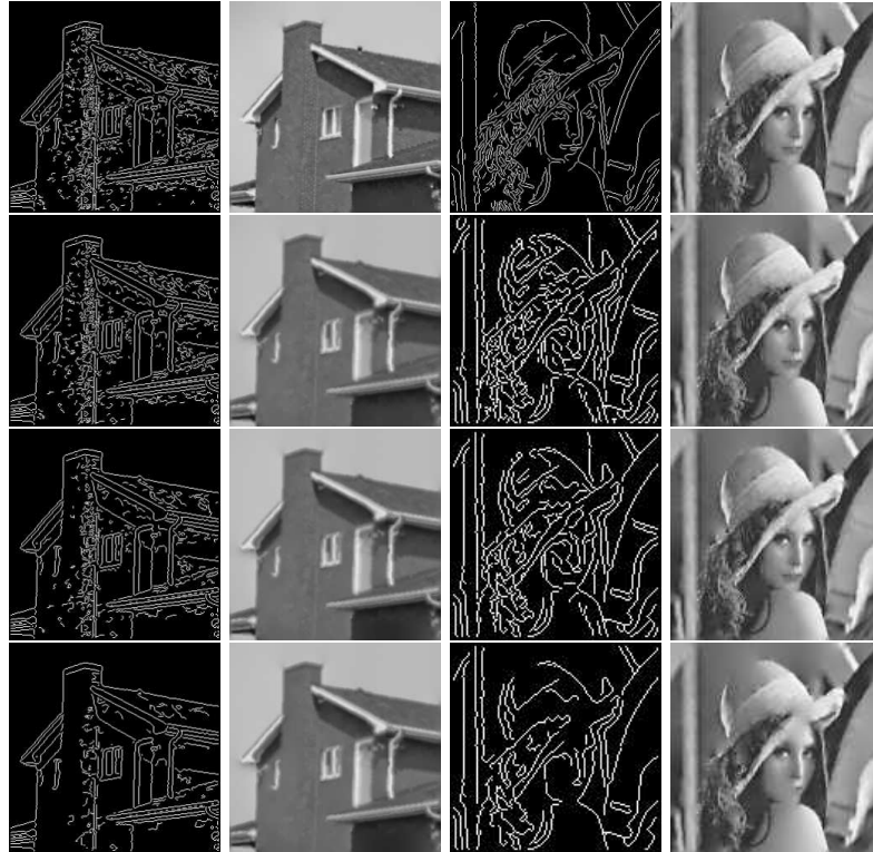
Figure 5. The selected edges and reconstructed images for House and Lenna images. From top to bottom, 100, 75, 50 and 25% of edges are retained.
