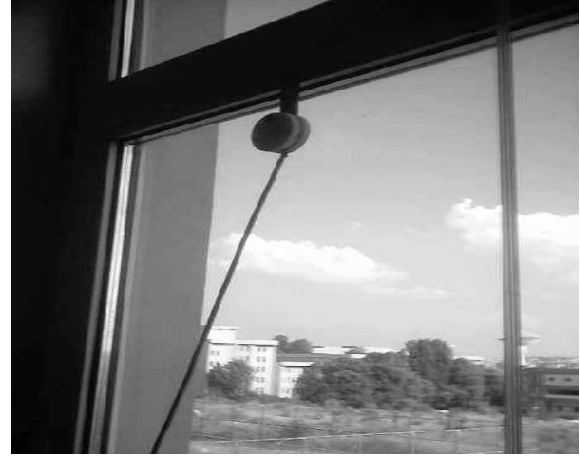
Figure 2. The unshielded sensor to measure the source illuminance.
