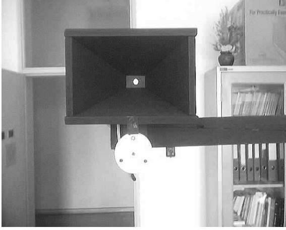
Figure 3. The shielded sensor inside a shield (not to see anything else but the window) to measure the window illuminance.
