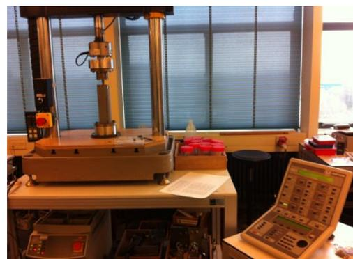
Fig. 14. Instron 8872 servo-hydraulic loading device.
